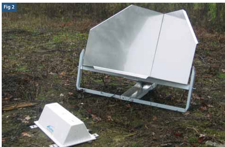
FIG. 2: Photograph showing artificial radar reflectors. The metallic structure is a Corner Reflector (CR) which reflects the radar signal back to the satellite. The smaller unit is a Compact Active Transponder (CAT), which offers additional facilities for point motion monitoring.
